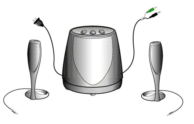
Connect the speaker system as shown in the **Connecting the speaker system to sound card** illustrations. Once the speaker system is properly connected, turn on the power switch located on the rear of the subwoofer.
