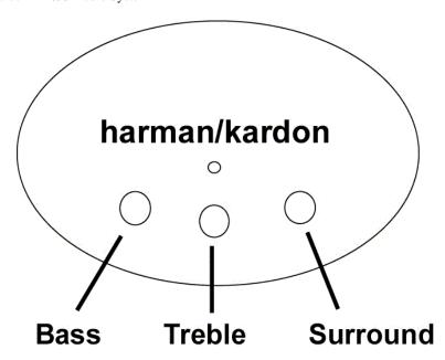
The are three tone and effects level knobs located on the top of the subwoofer. They control Bass, Treble and Surround.
